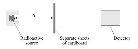
The detector measured the count rate for different numbers of sheets of cardboard. The distance  $\mathbf{X}$  was kept constant.
