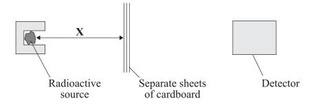
The detector measured the count rate for different numbers of sheets of cardboard. The distance X was kept constant.
