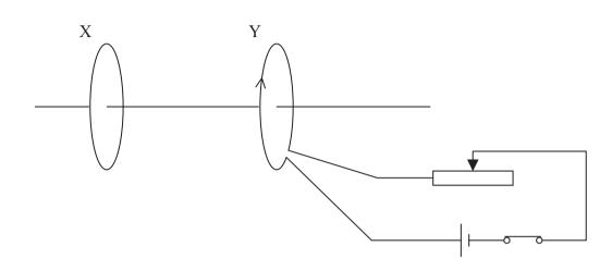
Coil Y is connected to a cell, a variable resistor and a closed switch.
