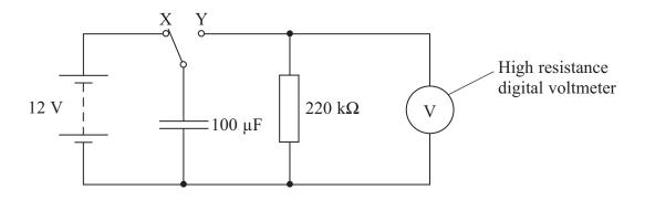
With the switch in position X the capacitor is charged to 12 V. When the switch is moved to position Y the capacitor discharges through the resistor and the potential difference (p.d.) across the resistor falls steadily from 12 V.
