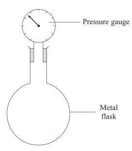
You are to plan an experiment to see how the pressure of the air in the flask varies with temperature.
