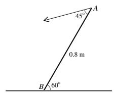
A uniform rod AB has weight 6N and length 0.8 m. The rod rests in limiting equilibrium with B in contact with a rough horizontal surface and AB inclined at  $60^{\circ}$  to the horizontal. Equilibrium is maintained by a force, in the vertical plane containing AB, acting at A at an angle of  $45^{\circ}$  to AB (see diagram). Calculate
