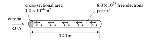
A current of  $8.0\,\mathrm{A}$  is passed through a conductor of length  $0.40\,\mathrm{m}$  and cross-sectional area  $1.0\times10^{-6}\,\mathrm{m}^2$ . The conductor contains  $8.0\times10^{28}$  free electrons per  $\mathrm{m}^3$ . When the conductor is at right angles to a magnetic field of flux density  $0.20\,\mathrm{T}$ , it experiences a magnetic force. What is the average magnetic force that acts on **one** of the free electrons in the wire?
