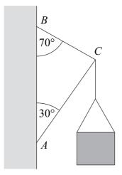
Find the magnitudes of the forces in rods AC and BC, stating whether the rods are in tension or compression. (7 marks)
