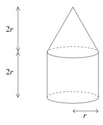
(i) Show that the centre of mass of the rocket is at a distance of  $\left(\frac{6+5k}{6+2k}\right)r$  from the base of the rocket. (5 marks)
