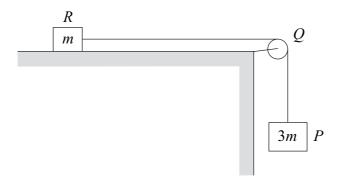
Model the pulley as a uniform disc of mass 12m and radius r. Model the blocks as particles.
