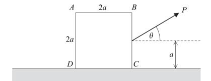
A force, of magnitude P, is applied at the mid-point of BC. This force acts in the plane ABCD and makes an angle  $\theta$  with the horizontal. The coefficient of friction between the cube and the plane is  $\mu$ .
